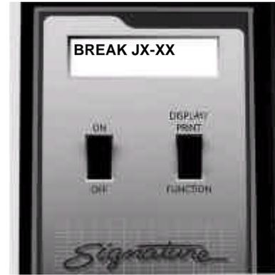
2. When you break a connection, the analyzer will prompt the next short. When all the shorts have been broken, the analyzer will prompt the net and point to which you should connect JX-XX. Connect JX-XX to the point indicated in the display.
