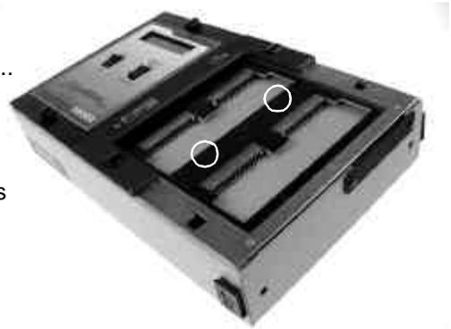
4. Lock the twistlock fasteners to hold the adapters firmly in place.
