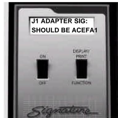
Installed adapters are not correct. Install correct adapters. When you've done that, prompt will change to **Ready to Test**.
