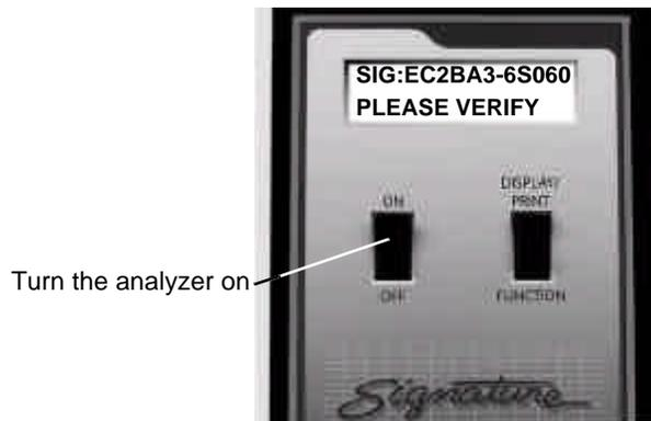
2. To verify that the Sample Cable has been learned correctly, press Display/Print.
